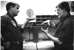
The P-19 engine is shown here running from the heat of the hand of astronaut David C. Burchdick on a recent visit to the University of Minnesota at Twin Falls. The reactor on the right is the heater. Unlike other Stirling engines we used, the P-19 easily runs at over 100 rpm when hand held. If the engine is placed on an insulated pad, it continues to run on the thermal energy in its warm plate for about 10 minutes.
